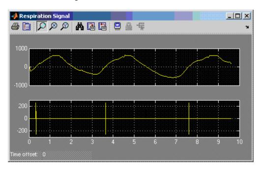
The **Respiration** display block shows the respiration cycles per minute.
