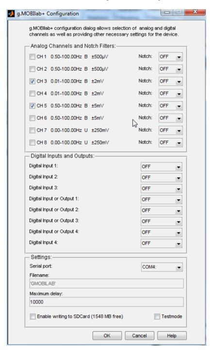
The check boxes for the analog channels (**CH 1** to **CH 8**) allow specifying the biosignal channels. Select channels 3 and 5 (**CH 3** and **CH 5**) to read in a DC channel with a lower cutoff frequency of 0. 01 Hz and an ECG channel.
