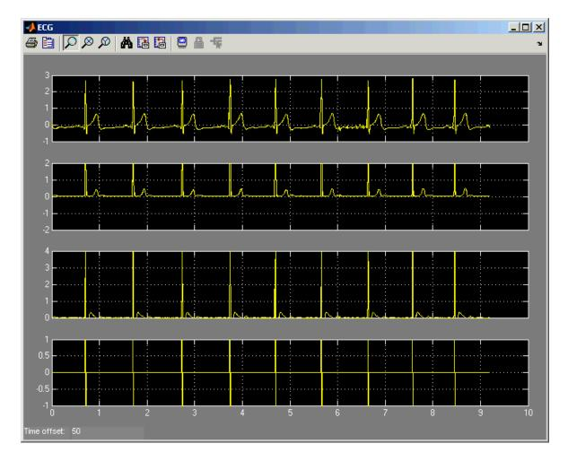
The block **ECG Detection** is a MATLAB S-Function that performs error detection of the QRS complex detector and of the respiration signal. Input 1 reads in the QRS complex signal and channel 2 the zero-crossings of the respiration channel.
